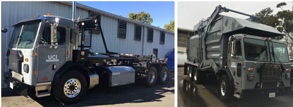
Left: New Compressed Natural Gas (CNG) Roll Off truck. Right: New CNG Front Loader truck.
